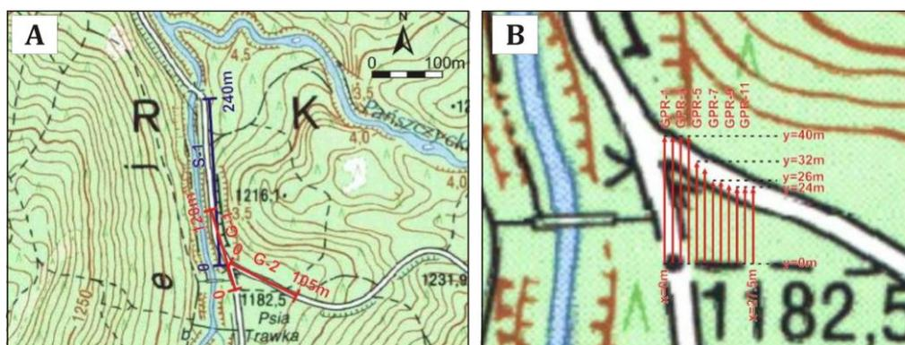
**Figure 1.** A) Profiles designed for 2D seismic and 2D GPR surveys with the use of 50 MHz antennae; B) Parallel profiles designed for 3D GPR surveys with the use of 100 MHz antennae (Backdrop: topographic map – [www.geoportal.gov.pl](http://www.geoportal.gov.pl)).
