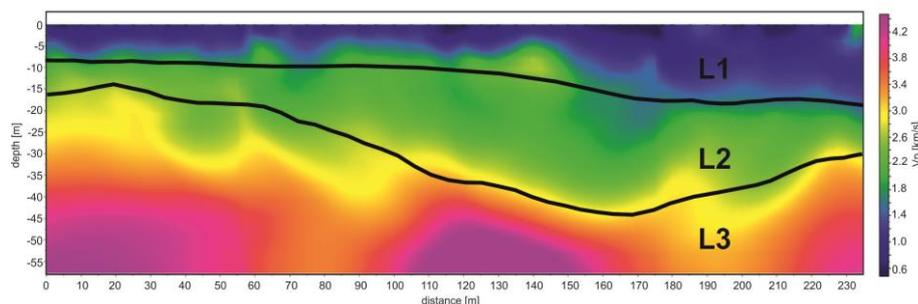
**Figure 3.** Seismic velocity imaging - tomographic solution. Solid lines - horizons interpreted by applying generalized reciprocal method, L1 - non compacted postglacial deposits, L2 - strongly compacted deposits, L3 – limestone.
