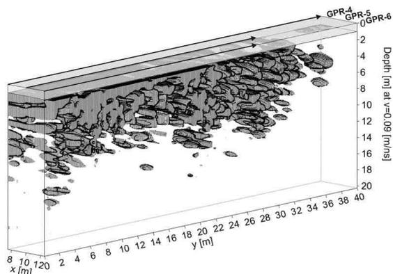
**Figure 2.** Results of 3D GPR surveys carried out along profiles from GPR-4 to GPR-6 (Fig. 1B), with the use of 100 MHz antennae. 3D visualisation was performed by outlying of the highest amplitudes of GPR signals – for this purpose Hilbert transform of signals and shading procedure were applied.
